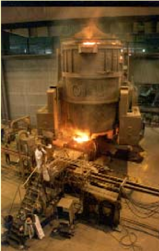
a 200T ladle during casting operations
