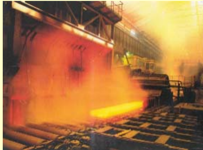
beginning of hot-rolling operations at 1200°C
