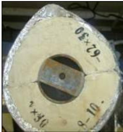
FIGURE 1 – End view of a Cyclic Pipe Test assembly showing the cross-sectional structure.
