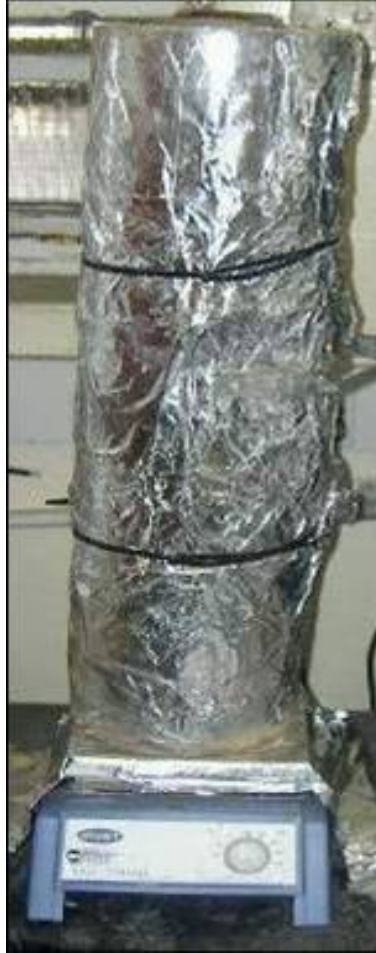
FIGURE 2 – View showing Cyclic Pipe Test Assembly placed on a hot plate for testing.
