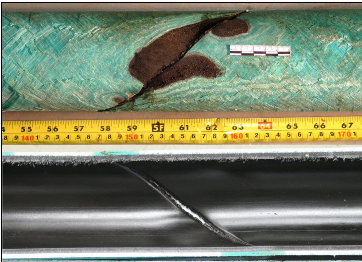
FIGURE 3 – Top Half External and Internal Surfaces: Area Of Failure
