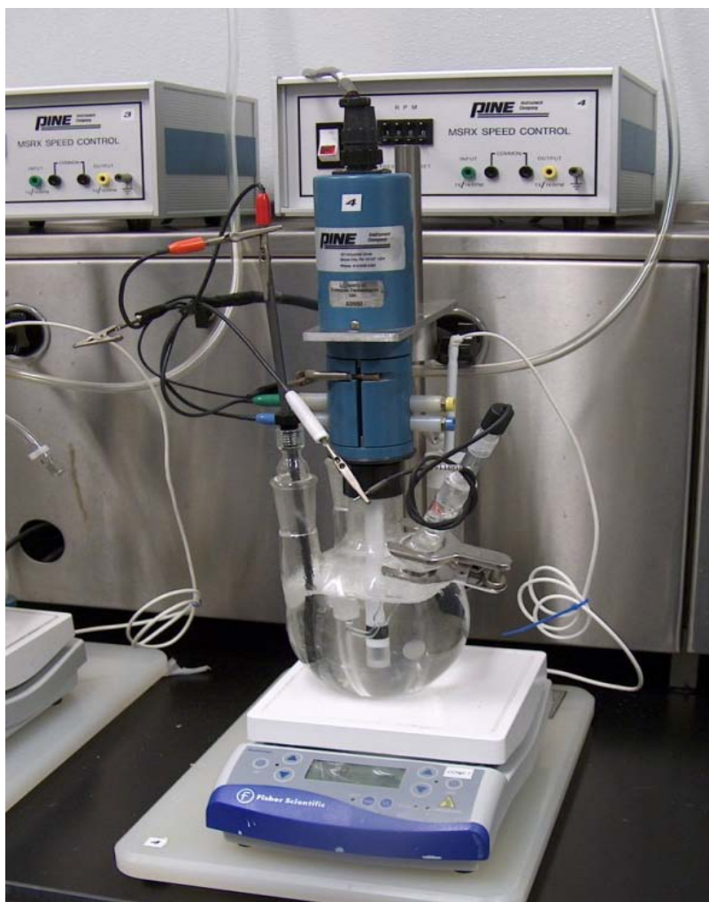
Figure 1: Rotating Cylinder Electrode Apparatus
