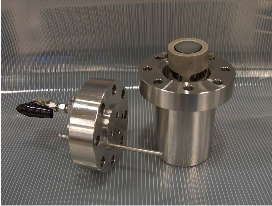
Figure 2: Static Autoclave Apparatus with Mushroom Cap Coupon
