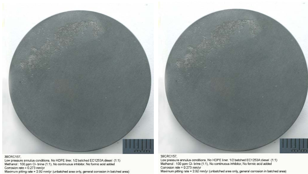
FIGURE 6 (left) - Surface morphology of a coupon exposed to low-pressure annulus conditions (Test # 5).
