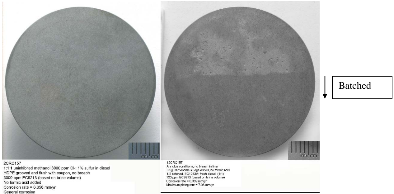
FIGURE 4 (left) - Surface morphology of a coupon exposed to pipeline conditions (Test #1)
