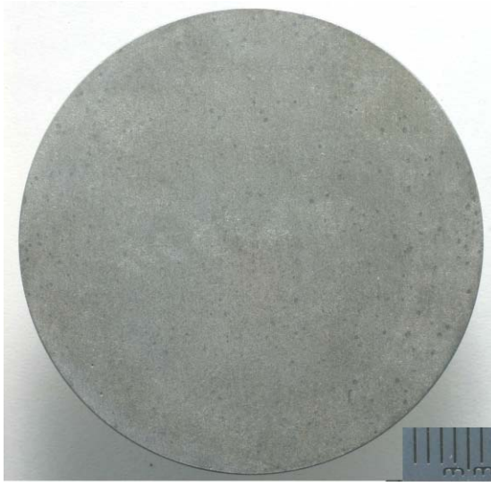
3CRC157 1:1:1 uninhibited methanol:8000 ppm Cl - : 1% sulfur in diesel HDPE grooved with space between coupon and liner, breach in the liner 3000 ppm EC9213 (based on brine volume) No formic acid added Corrosion rate = 0.413 mm/yr Maximum pitting rate = 4.02 mm/yr
