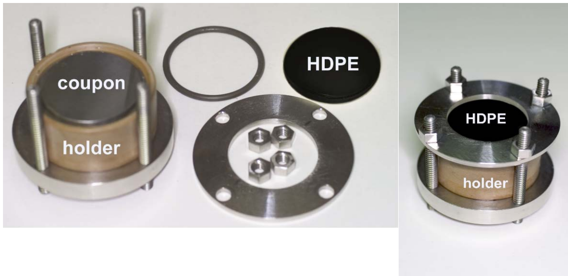
FIGURE 3 - Setup used for corrosion tests in which HDPE was placed on the top of carbon steel surface
