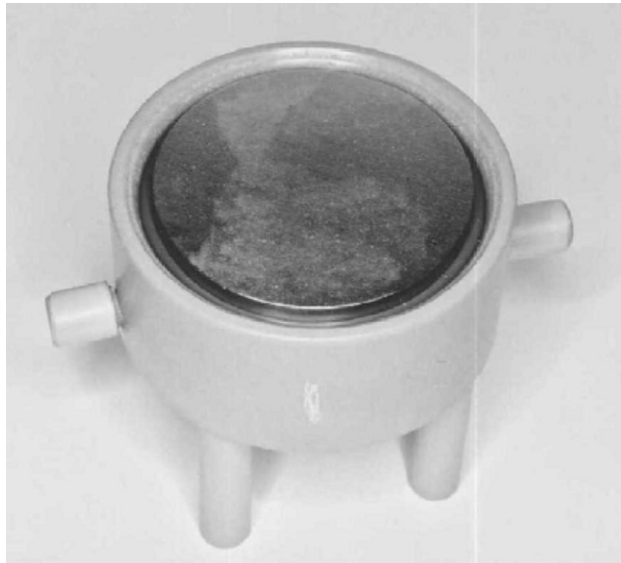
FIGURE 2 - Bare Corrosion Coupon in Holder
