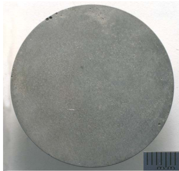
4CRC157 1:1:1 uninhibited methanol: 8000 ppm Cl - : 1% sulfur in diesel HDPE grooved with space between coupon and liner, breach in the liner 3000 ppm EC9213 (based on brine volume) 1000 ppm formic acid added Corrosion rate = 0.420 mm/yr Maximum pitting rate = 21.1 mm/yr
