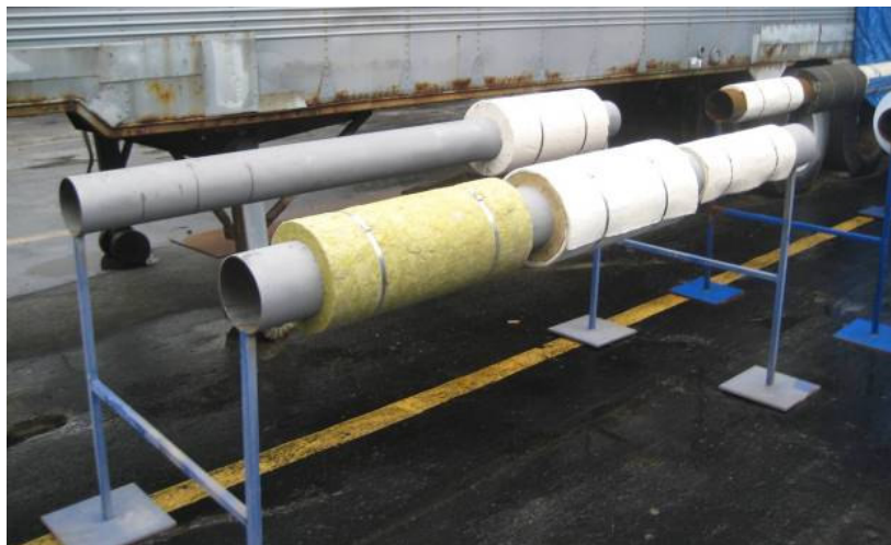
Figure 15: Outdoor pipe stands with the various insulation test sections.
