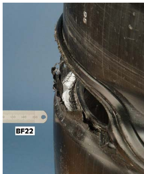
Figure 14 Photograph showing the fracture of a weld made under Condition 2.
