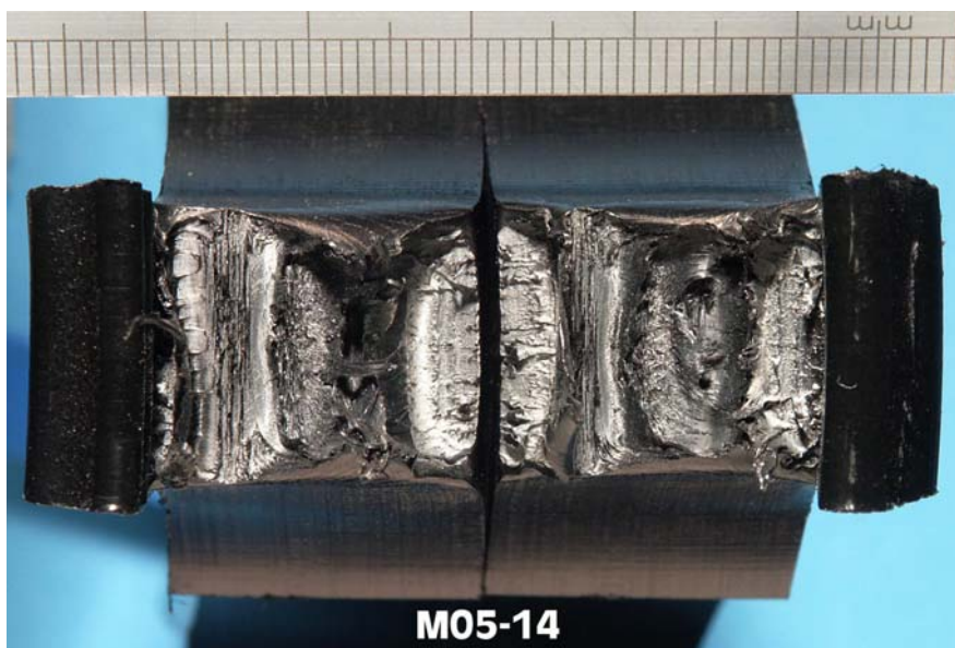
Figure 12 Fracture surface of creep rupture test specimen welded under Condition 2.
