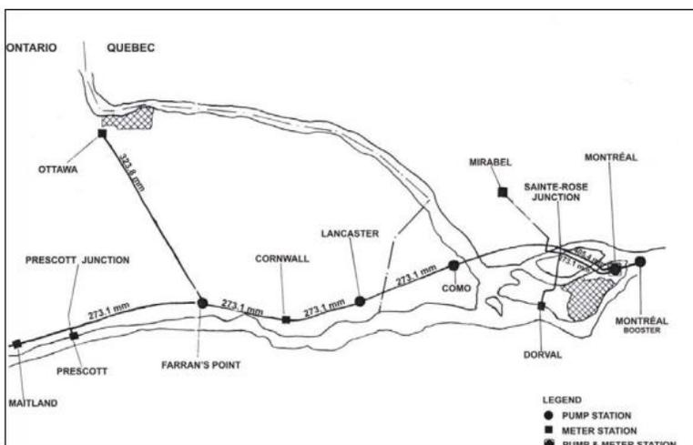
Schematic of the Trans-Northern Pipelines Inc. Pipeline System from the Montréal Pump Station to the Ottawa Terminal
