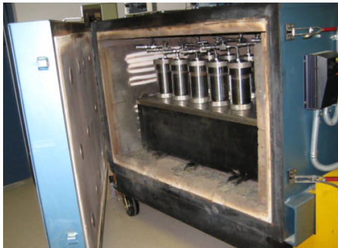
Figure 2 Stirred Autoclave Test in High Temperature Oven
