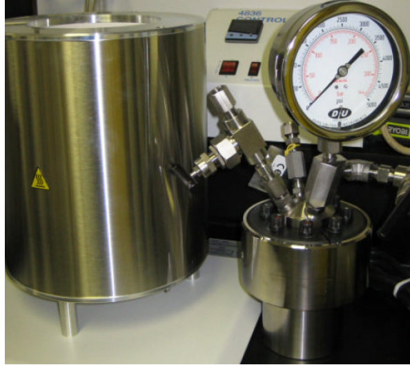
Figure 3 High Temperature and Pressure Hastelloy Autoclave
