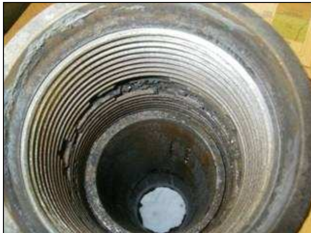
FIGURE 8 - Internal corrosion of coupling area of downhole tubing (Female Connector)
