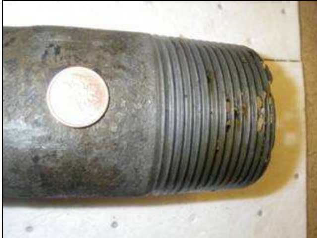
FIGURE 9 - External view of corroded threaded area of downhole tubing (Male connector)
